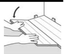
5. Push a laying wedge in under the end of the board already laid.
