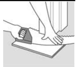
14. The last row of boards must be cut to the correct width.
